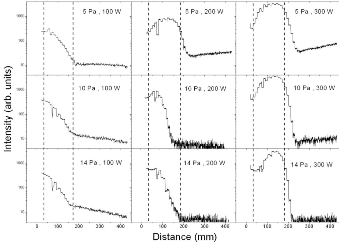
Figure 1: Spectral intensities along plasma vessel tube of the OH emission at 309 nm. Vapour flow is from the left to right. Vertical dashed lines indicate position of the coil.
